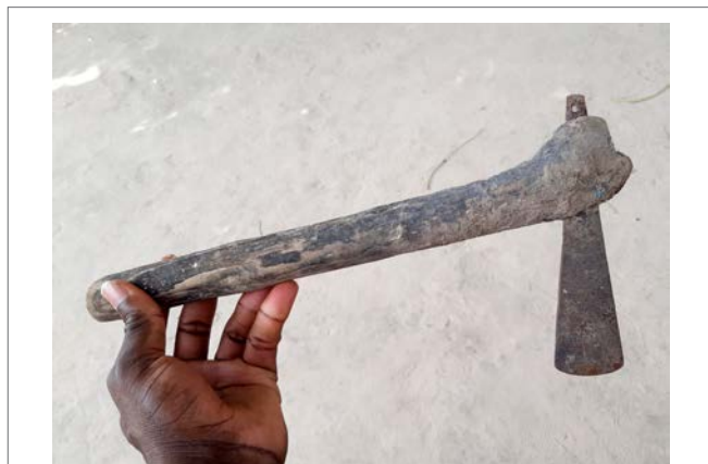
FIGURE 7 | Specialized mini axe (hatchet) used for harvesting oysters from mangrove roots without cutting the mangroves. [Data source: Image captured by authors for this study].
