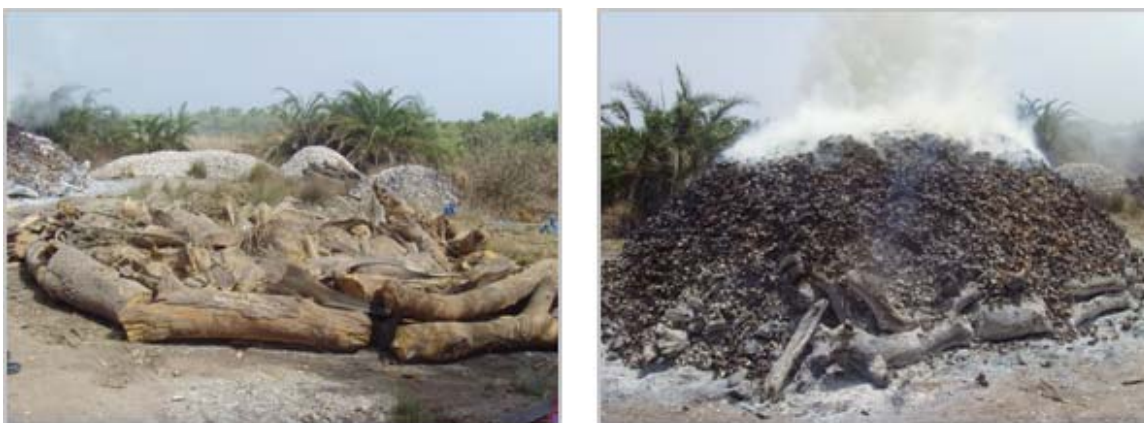
Fig. 28: Lime production setup with tree logs bedding (left) and burning shells during production process
