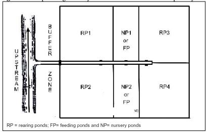
Figure 2. Sample design and layout of a conventional milkfish pond system
