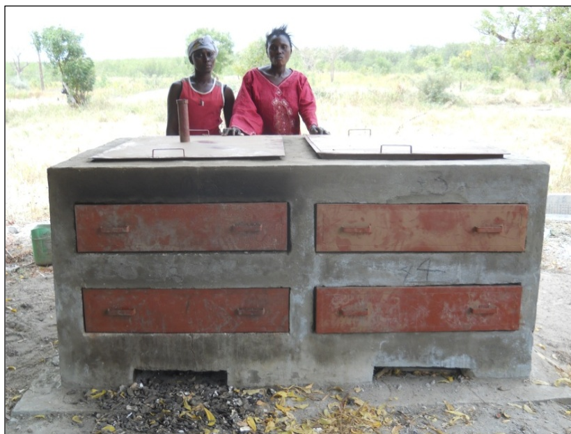
Figure 6: Oyster smoking oven technology transferred from Senegal, constructed at Kamalo oyster site.
