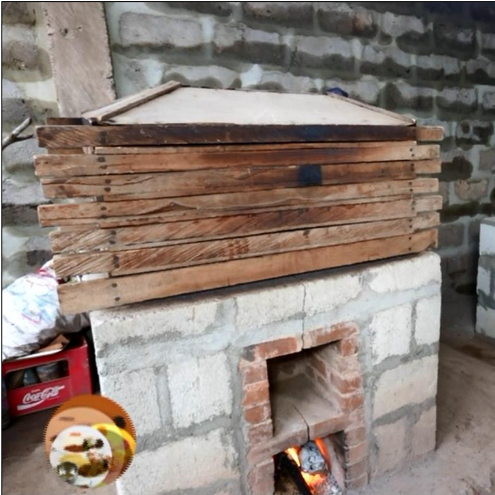
Figure 19. The newly developed fish-smoking technology – the Ahotor oven
