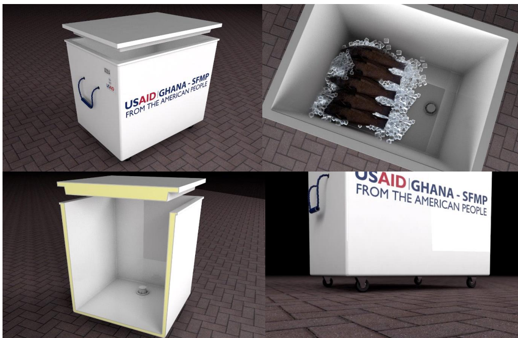
Figure 2. Three-dimensional view of the insulated containers
