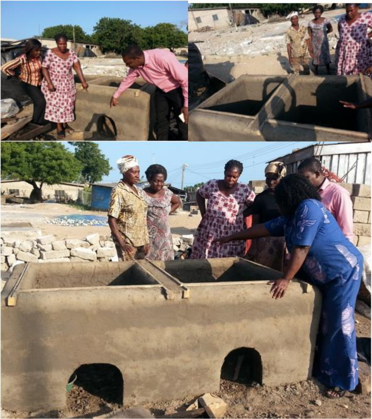
Figure 1. Inspection of Constructed Morison Oven in Winneba, in the Central Region of Ghana
