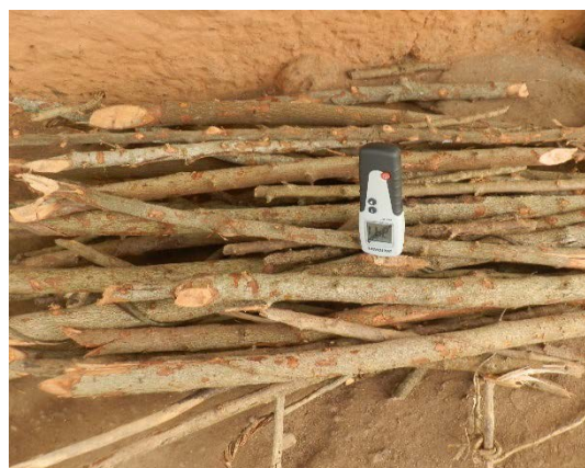
Figure 3: Measurement of woodfuel moisture content
