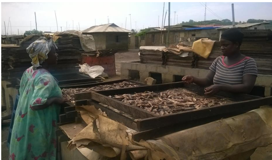
Plate 2 Fish processing using chokor smoker – Apam Community
