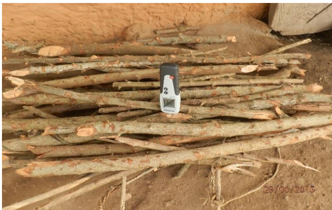
Figure 3 Measurement of woodfuel moisture content
