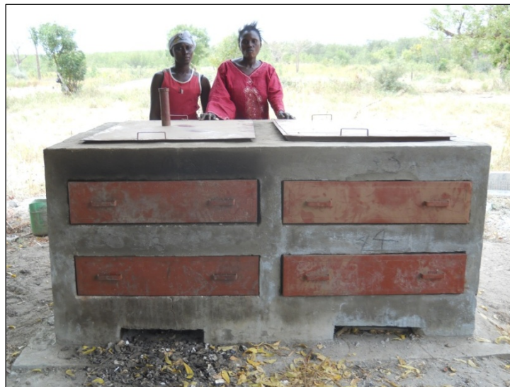
Figure 5: Oyster smoking oven technology transferred from Senegal, constructed at Kamalo oyster site.
