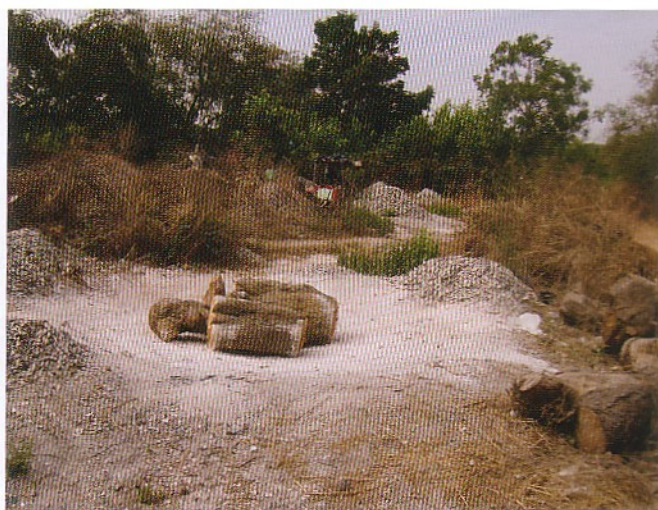
Fig. 7. Small-scale lime production operation in Kartong, Gambia. Empty shells of locally harvested blood ark clams are burnt using wood fires to manufacture lime for masonry mortar and other uses. Photo by Michael A. Rice.
