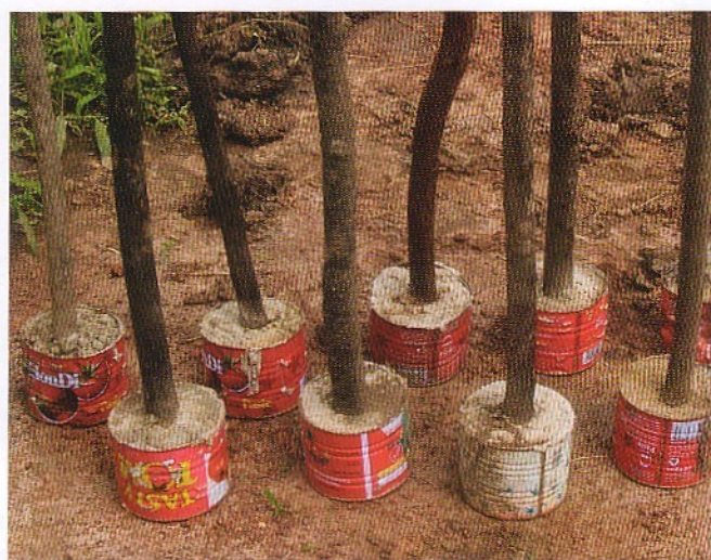
Fig. 3. Manual soil compactors constructed with sticks held in concrete poured into 4-L metal cans. Photo by Famara Darboe.
