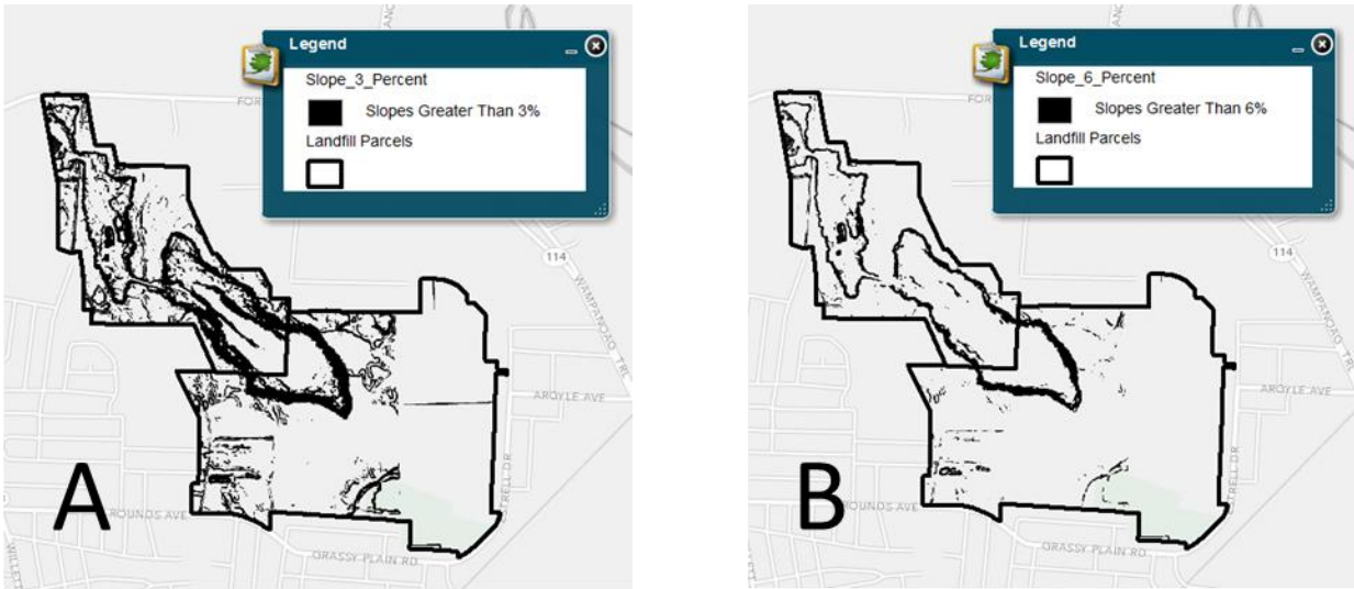
Figure 6. A) Slopes Greater than 3%; B) Slopes Greater than 6% (Forbes St. Landfill, East Providence)
