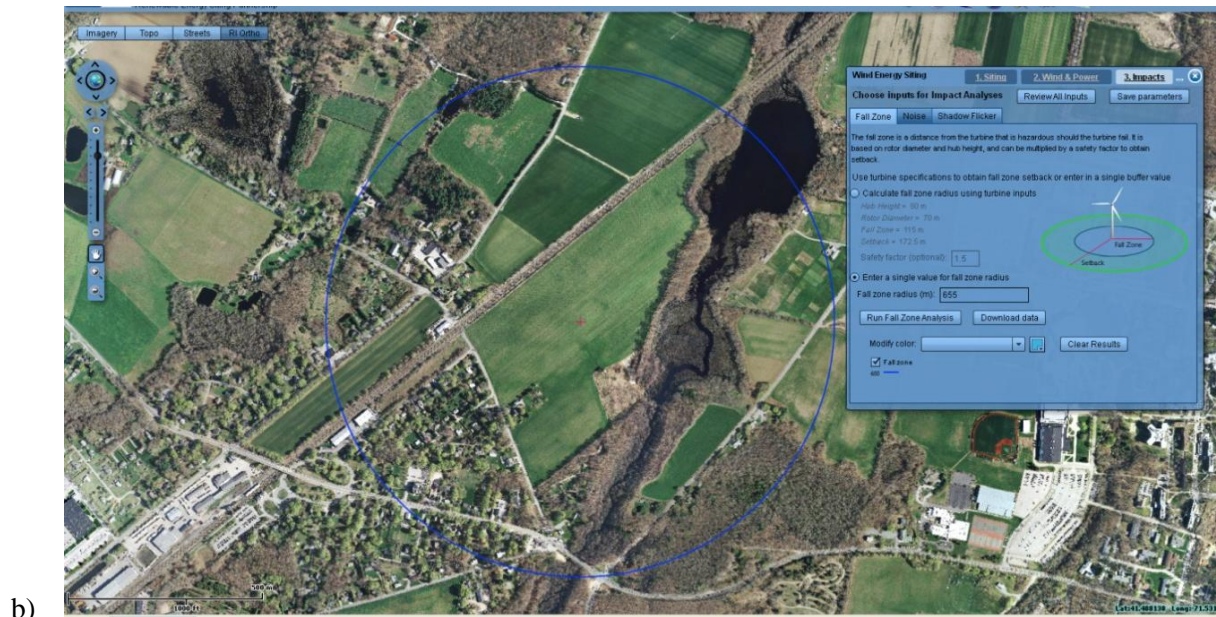
Ch. 4 Figure 5. Fall Zone Setbacks (a) based on the height of the turbine specified (e.g. 1.5* Total Turbine Height); (b) Setback based on a certain radius (e.g. distance calculated by methodology described in the Wind Chapter conducted by Rogers et al. (2011)).
