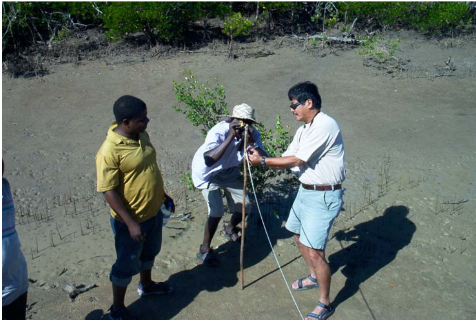
Volunteer Edwin Requentina demonstrating the method of determining low tide baseline elevation datum, tide range determination, and the method for transferring tide measurements to make proper dike and pond bottom elevations
