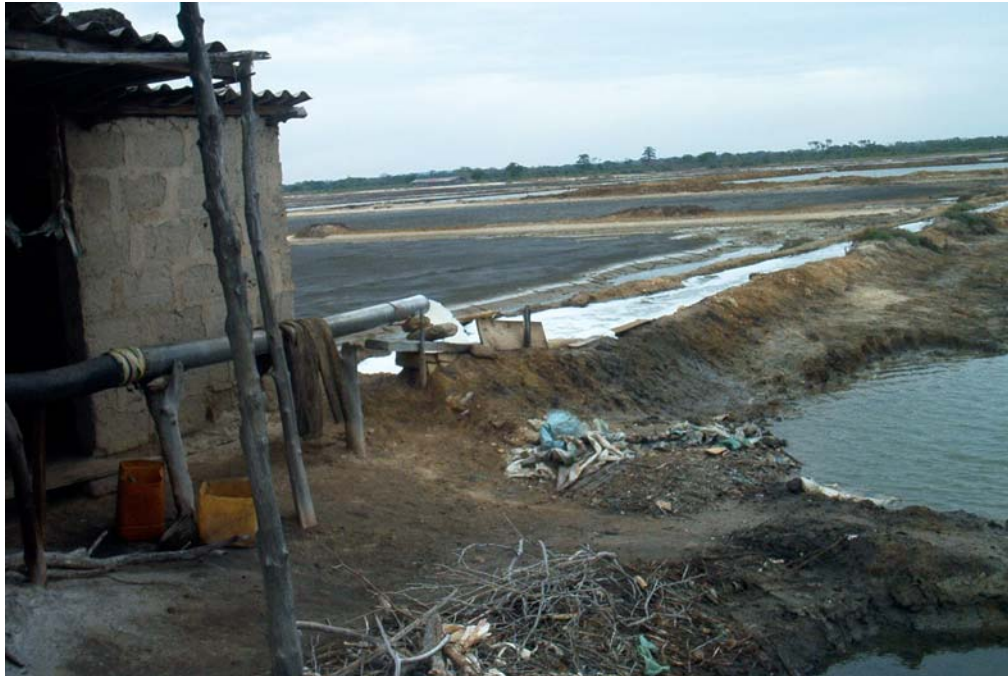
Water is pumped into high salt pans by diesel engine driven centrifugal pump at Regent Enterprises salt pans
