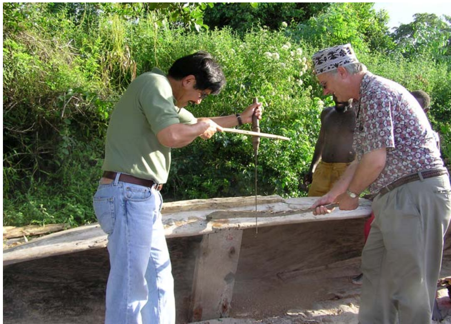
Volunteers Requentina and Rice learn the technique of the traditional bow drill from a Bagamoyo boat builder
