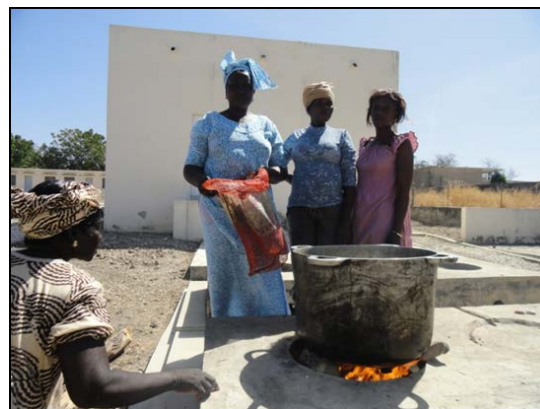
Figure 12 and Figure 13. Cockles are put in a mesh bag and the bag put in a large cooking pot (property of the plant), then placed over a fuel efficient stove to steam the cockles.
