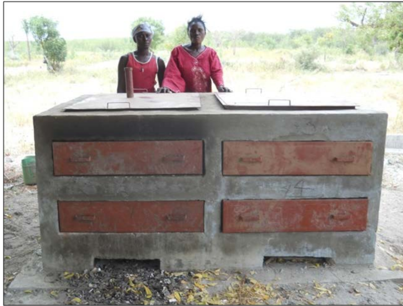
Figure 6. Fuel saving oyster smoking oven demonstrated at Kamalo oyster harvesting site with USAID/BaNafaa support in FY12 now replicated at 15 TRY oyster harvesting sites with UNDP funding.
