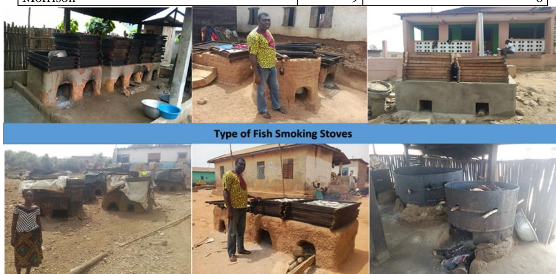
Figure 9 Gallery of Types Fish Smoking Stoves Currently being used by Smoked Fish Processors
