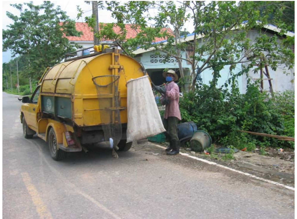
Figure 7. A 6-m 3 truck for solid waste collection in Tambon Kampuan
