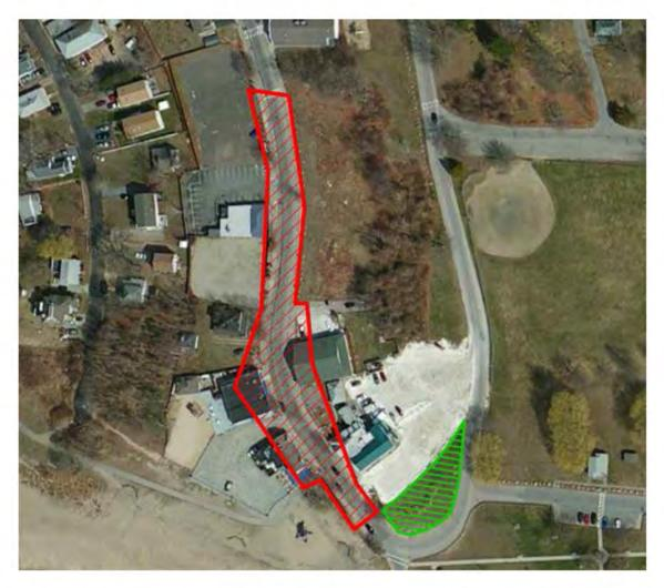
The stormwater runoff from the watershed is captured in the proposed bioretention basin and pollinator meadow.
