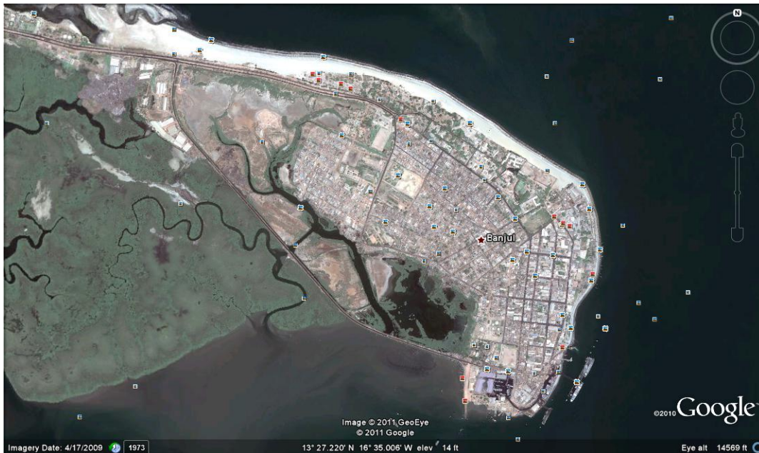
Figure 3. Satellite imagery of Banjul showing the Bund Road Levee and associated drainage area in metropolitan Banjul.
