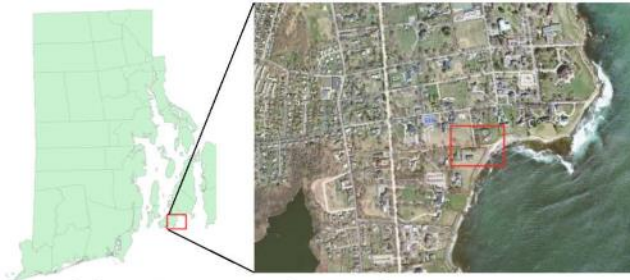
The stormwater runoff from the watershed (275,000 sqft, 6.3 acres) is captured in the proposed bioretention basin, see Appendix X for sizing information
