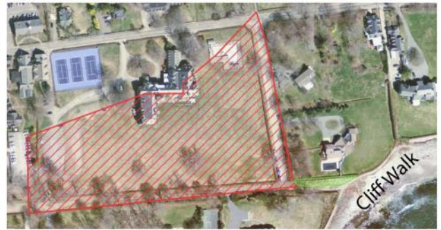
The stormwater runoff from the watershed (275,000 sqft, 6.3 acres) is captured in the proposed bioretention basin, see Appendix X for sizing information
